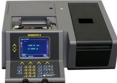
A photograph of a UV-VIS spectrophotometer model Genesys 2 by Spectronic. The device consists of a central control unit with a color touchscreen display and a keypad, flanked by two dark, rectangular components, likely the light source and detector assembly.                                          |
