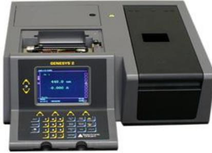
A photograph of a UV-VIS spectrophotometer. It consists of a central control unit with a color touchscreen display showing spectral data and a keypad, flanked by two dark, rectangular components representing the light source and detector assembly.                                                     |
